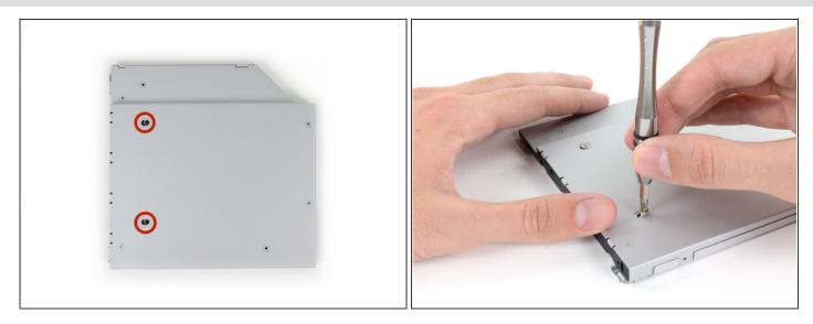
• Use two Phillips #1 screws to secure the drive to its enclosure.
